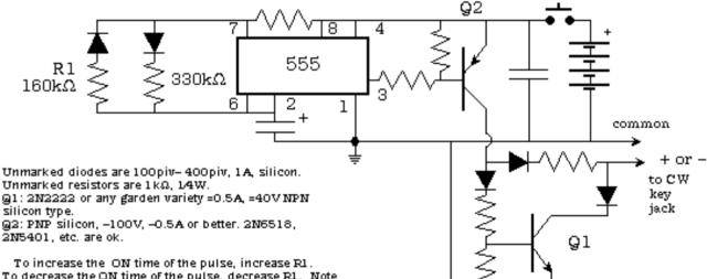
To increase the ON time of the pulse, increase R1. To decrease the ON time of the pulse, decrease R1. Note that the position of R1 is reversed in the two diagrams. This is due to the effect of Q2 which inverts the 555's output pulse in the circuit that is capable of switching positive or negative voltages.
