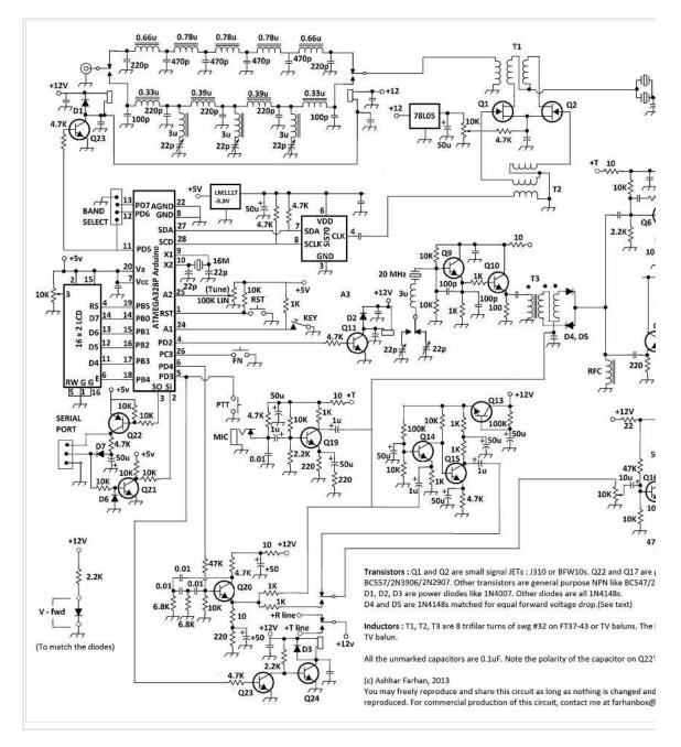
The Minima architecture is slightly different from that of a traditional superhet transceiver.
