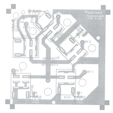
RA-20A-2 ANTENNA SWITCH CONTROL ASSEMBLY RA20A200 COMPONENT LOCATOR VIEWED FROM COMPONENT SIDE (FOIL APPEARS AS VIEWED THRU BRD) SCALE 1:1 2.375" X 4.375" FLAG TO FLAG JLK 11-21-11 REV 0
